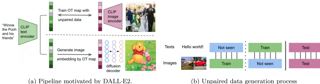
Figure 3: (a) During the training process (above the dotted line), our map learns to generate image embeddings that maximize the expected similarity with input texts. During the evaluation (below the dotted line), given a text encoding from the CLIP model, our map outputs an image embedding, which conditions a pre-trained diffusion decoder to generate an image. The CLIP encoder and diffusion decoder are both pre-trained and frozen.
